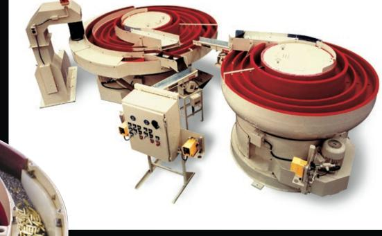
The Multi-Pass® machine can also operate as a continuous process machine using part to media ratios used in conventional processes. The example shown at left is producing 1,400 pieces per minute continuously.
