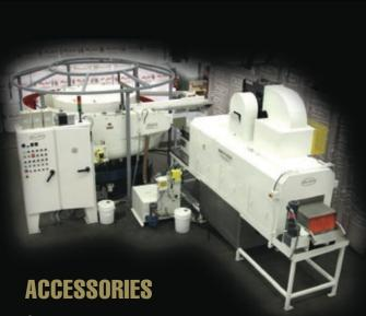
Other available features for the Multi-Pass® are a Gazebo Sound Cover (frame pictured) for noise reduction and an External Parts Washer.
