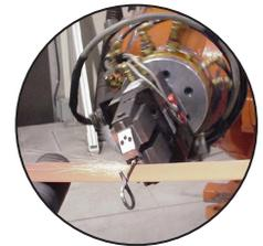
Formed Gripper for Small Parts
