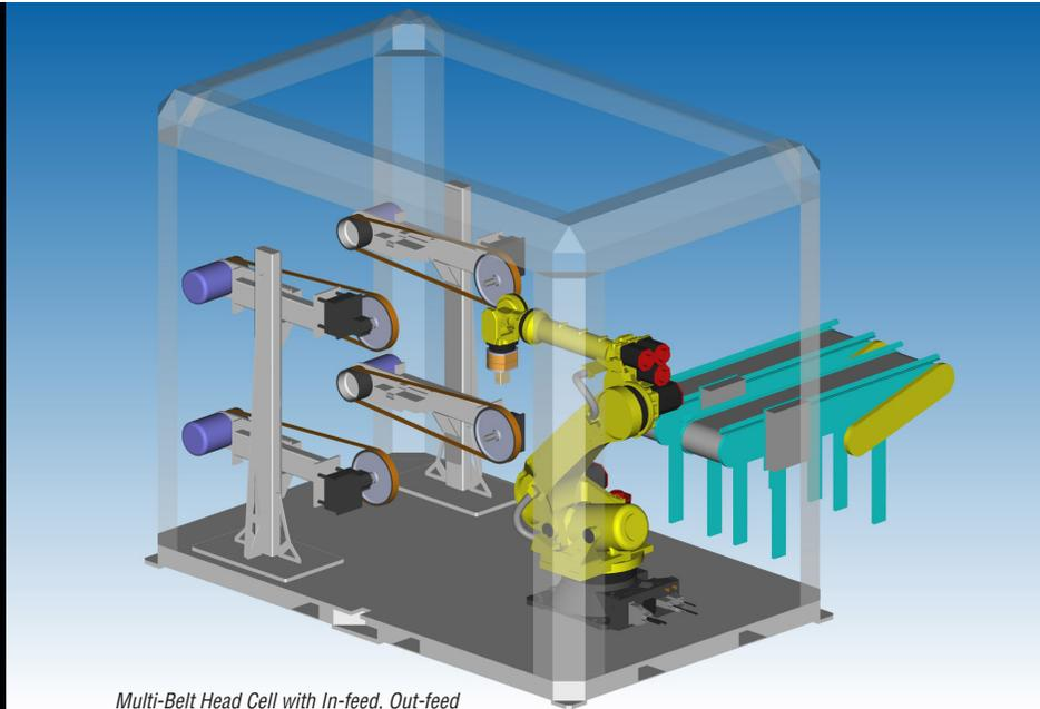
Multi-Belt Head Cell with In-feed, Out-feed
